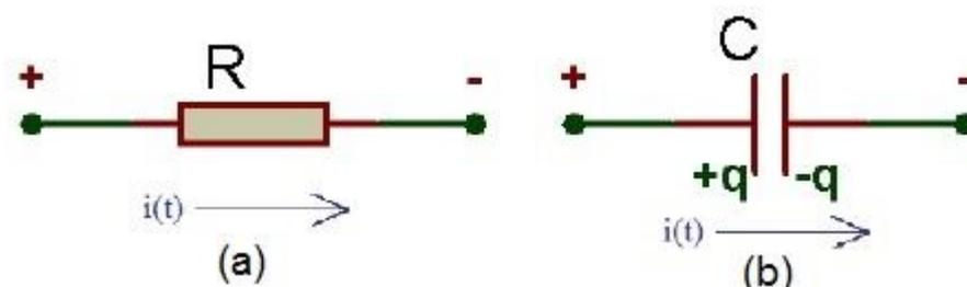
Figura (1): (a) Resistor; (b) Capacitor.
