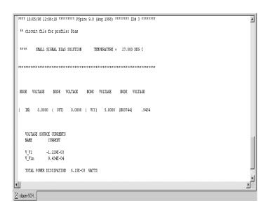
Figure 5 Simulation output file.
