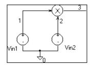
Figure 54 *Voltage multiplier circuit* (mixer).
