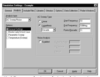
Figure 19 AC sweep and noise analysis simulation settings.
