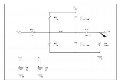
Figure 8 Clipper circuit with voltage marker on net Out.
