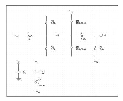
Figure 14 *Diode clipper circuit with a voltage stimulus.*
