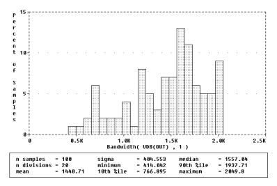
Figure 82 1 dB bandwidth histogram.
