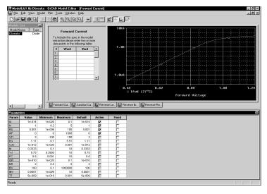
Figure 31 Model characteristics and parameter values for DbreakX.
