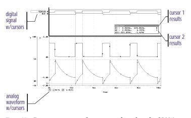
Figure 97 Cursors positioned on a trough and peak of V(1)
