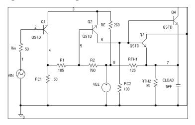
Figure 65 ECL-compatible Schmitt trigger.
