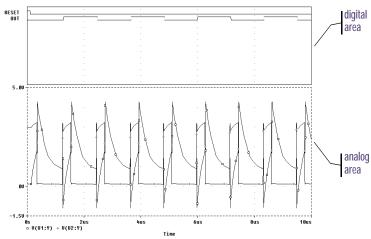
Figure 91 Analog and digital areas of a plot.
