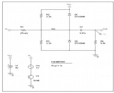
Figure 22 Clipper circuit with global parameter Rval.
