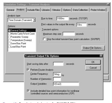
Figure 63 Transient analysis setup for EXAMPLE.OPJ.
