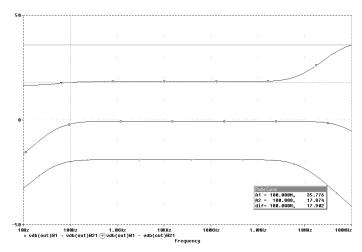
Figure 25 Small signal frequency response at 100 and 10  $k\Omega$  input resistance.
