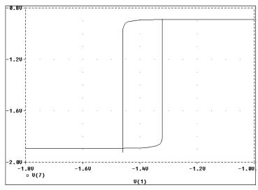
Figure 67 Hysteresis curve example: Schmitt trigger.
