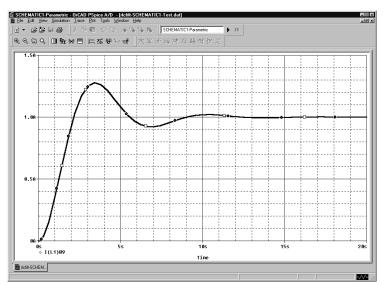
Figure 69 Current of L1 when R1 is 1.5 ohms.
