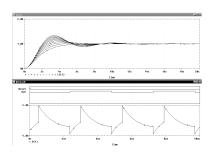
**Perform post-simulation analysis of the results** This means you can plot additional information derived from the waveforms. What you can plot depends on the types of analyses you run. Bode plots, phase margin, derivatives for small-signal characteristics, waveform families, and histograms are only a few of the possibilities. You can also plot other waveform characteristics such as rise time versus temperature, or percent overshoot versus component value.
