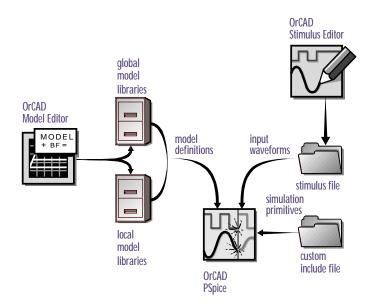
Figure 1 User-configurable data files that PSpice reads
