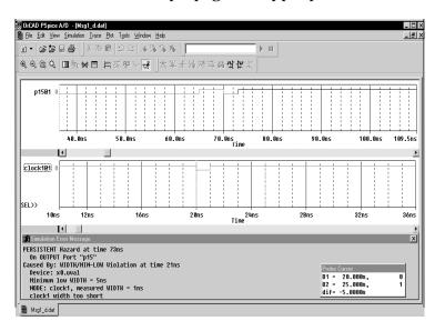
Figure 98 Waveform display for a persistent hazard.
