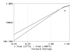
Figure 33 Forward Current device curve at two temperatures.
