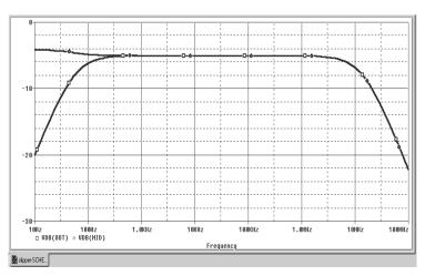
Figure 20 dB magnitude curves for "gain" at Mid and Out.
