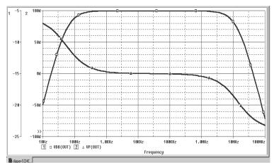
Figure 21 Bode plot of clipper's frequency response.
