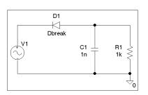
Figure 30 Design for a half-wave rectifier.
