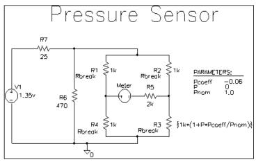
Figure 78 Pressure sensor circuit.
