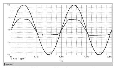
Figure 17 Sinusoidal input and clipped output waveforms.
