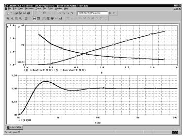
Figure 70 Rise time and overshoot vs. damping resistance.
