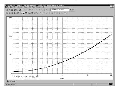
Figure 72 Plot of capacitance versus bias voltage.
