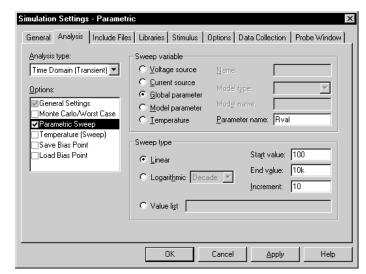
Figure 23 Parametric simulation settings.
