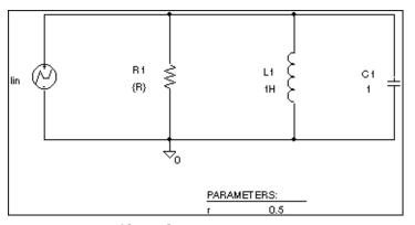
Figure 68 Passive filter schematic.
