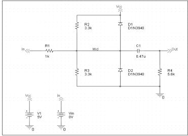
Figure 2 Diode clipper circuit.
