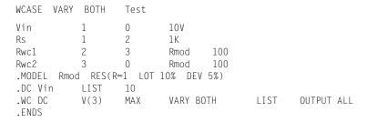
Figure 90 Circuit file using VARY BOTH.
