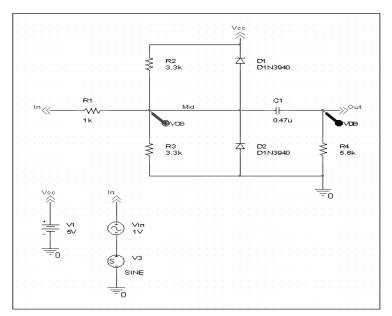
Figure 18 Clipper circuit with AC stimulus.
