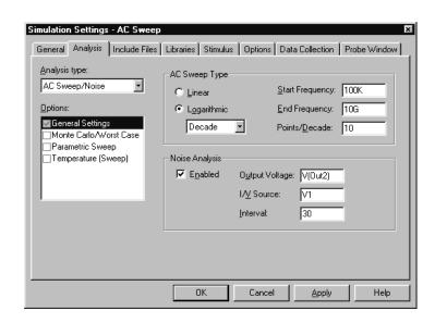
Figure 61 AC analysis setup for EXAMPLE.OPJ.
