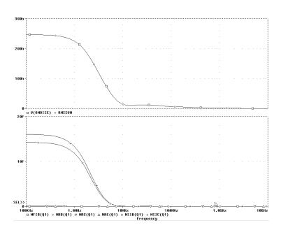
Figure 62 Device and total noise traces for EXAMPLE.DSN.
